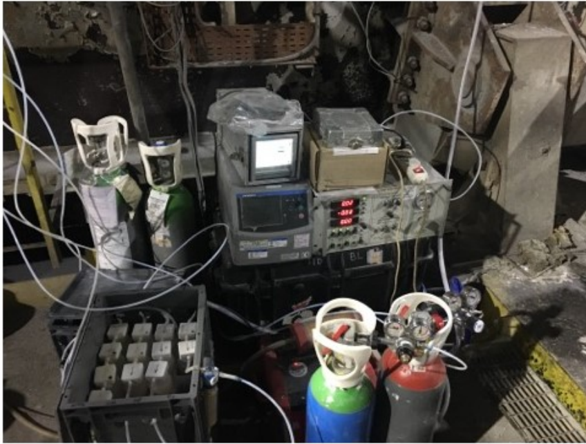
Figure 3. Equipment installed on top of the furnace to measure atmospheric emissions.
